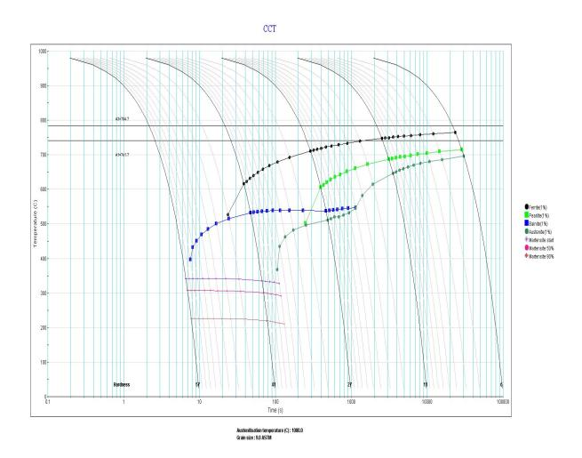
Calculated CCT diagram for the AISI 4140 steel.
